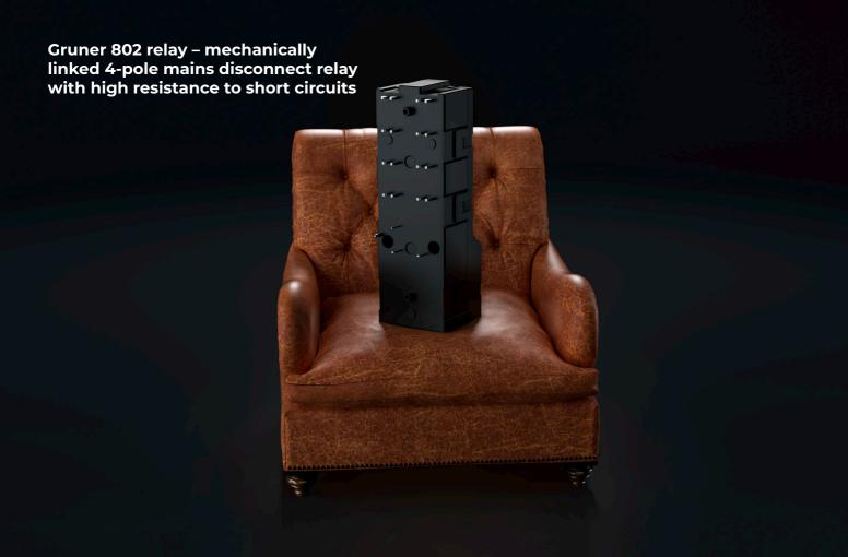
In accordance with the requirements of IEC 62955, Gruner has developed a 4-pole relay with mechanical coupling. The Gruner Relay 802 ensures that all poles are either closed or open and reduces the total number of relays and actuators required. This allows significant savings in components, energy and costs. In addition, Relay 802, which is designed for AC charging of electric vehicles up to 22 kW and has a
